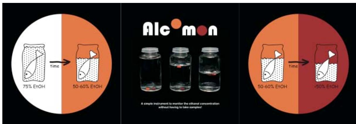
For these reasons, the so-called Alcomon Indicator System has been developed; an instrument that monitors the ethanol concentration in fluid preserved specimens and therefore eliminates the need to perform time-consuming conventional density measurements.
