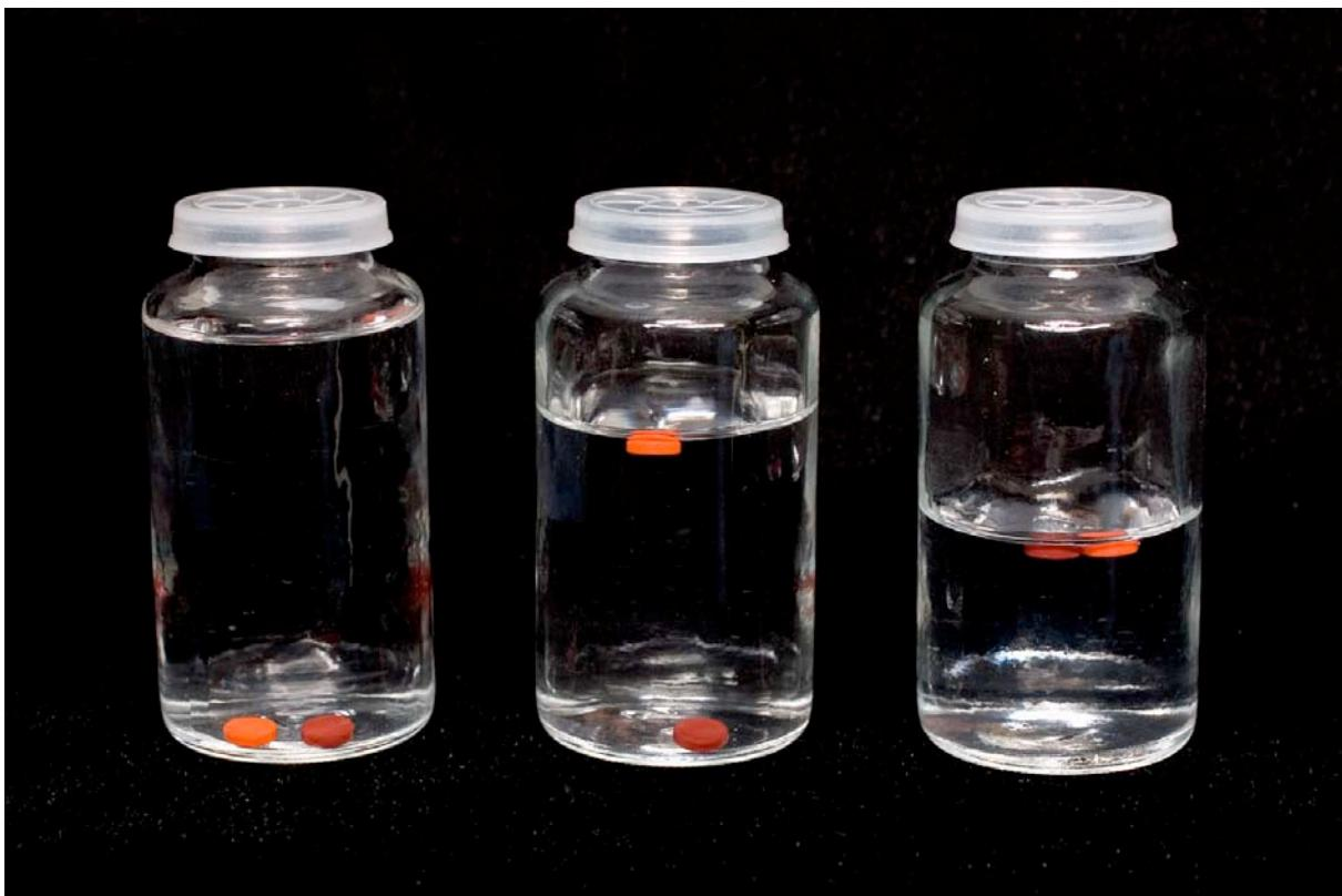
Starting with a freshly filled jar with 70 % ethanol both indicators will be on the bottom of the jar. After a certain time we discover that in several jars one indicator floats. This tells us that in these jars the ethanol concentration has dropped to a concentration between 50 and 60%. We know that the preservation strength of the fluid is still sufficient, which means that there is no immediate threat to the specimen.
